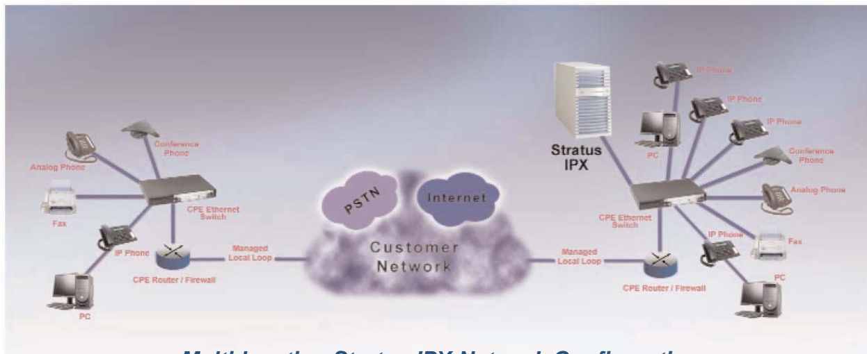
Multi-location Stratus IPX Network Configuration
